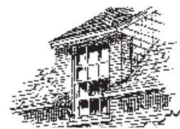
Shed roof dormer
