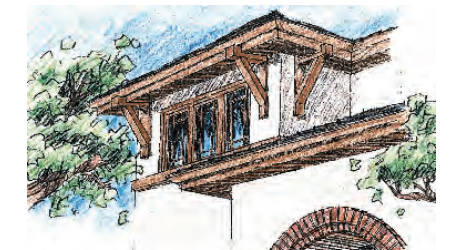
Knee braces supporting extended roof overhang
