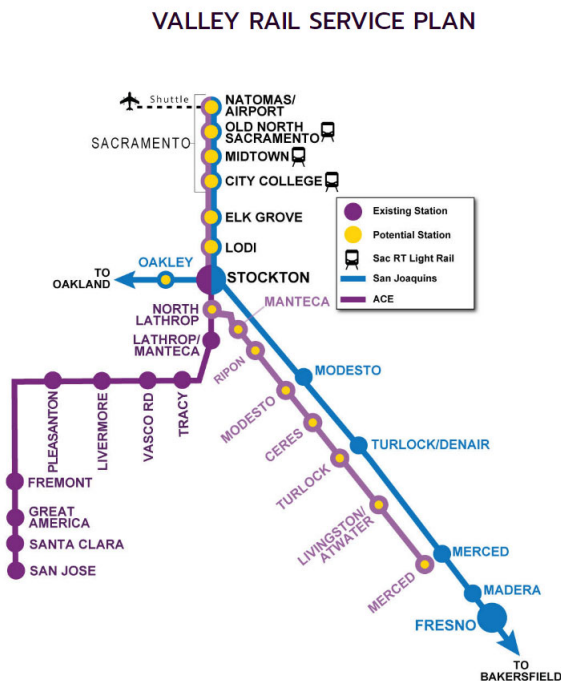
Figure 3-2 Valley Rail Existing and Future Service Plan
